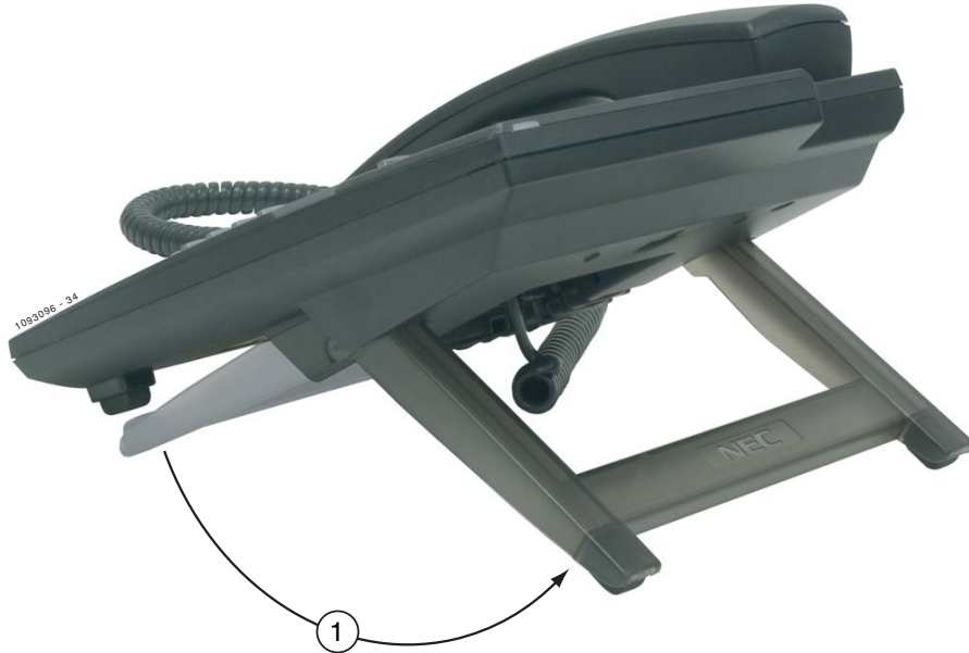
Figure 28: Setting the Low Viewing Angle
