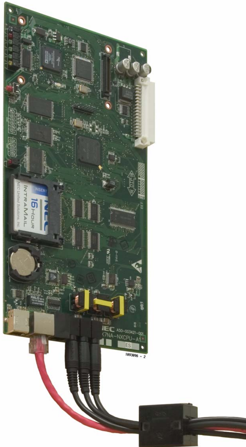
Figure 10: Installing the RFI Suppressor Assembly
