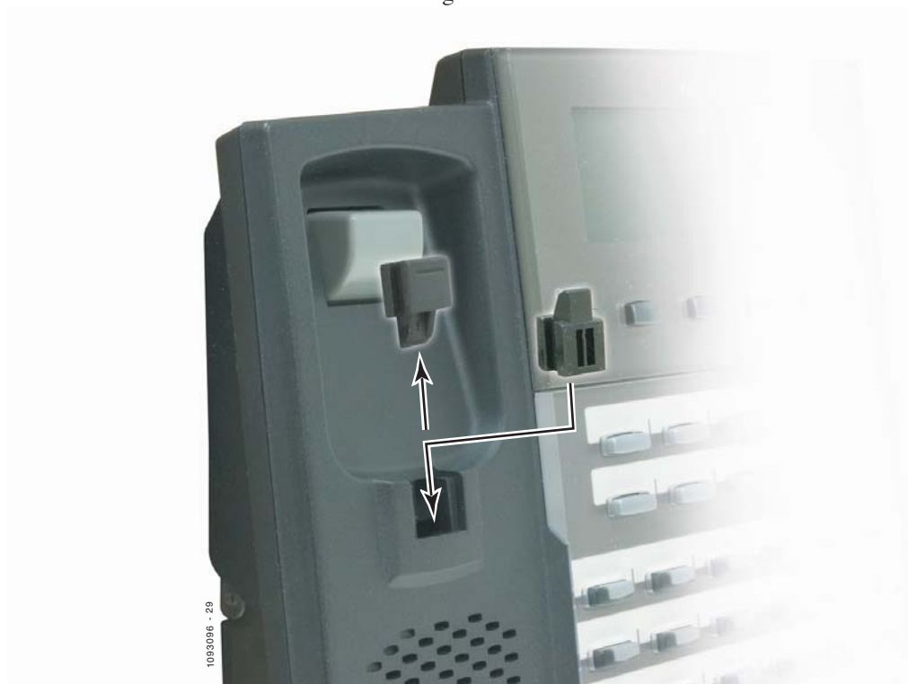
Figure 49: Reversing the Handset Hanger
