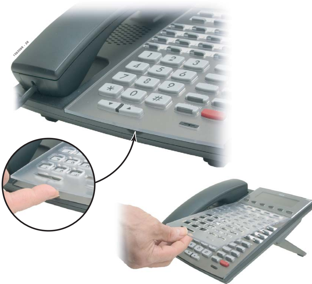
Figure 30: Removing the Telephone Faceplate
